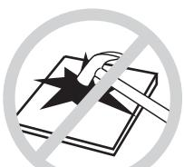
If the surface of the hob is cracked, switch off the appliance to avoid any possibility of electric shocks.
