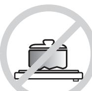
Do not place rough or uneven vessels on the hob, as they may damage the ceramic surface.
